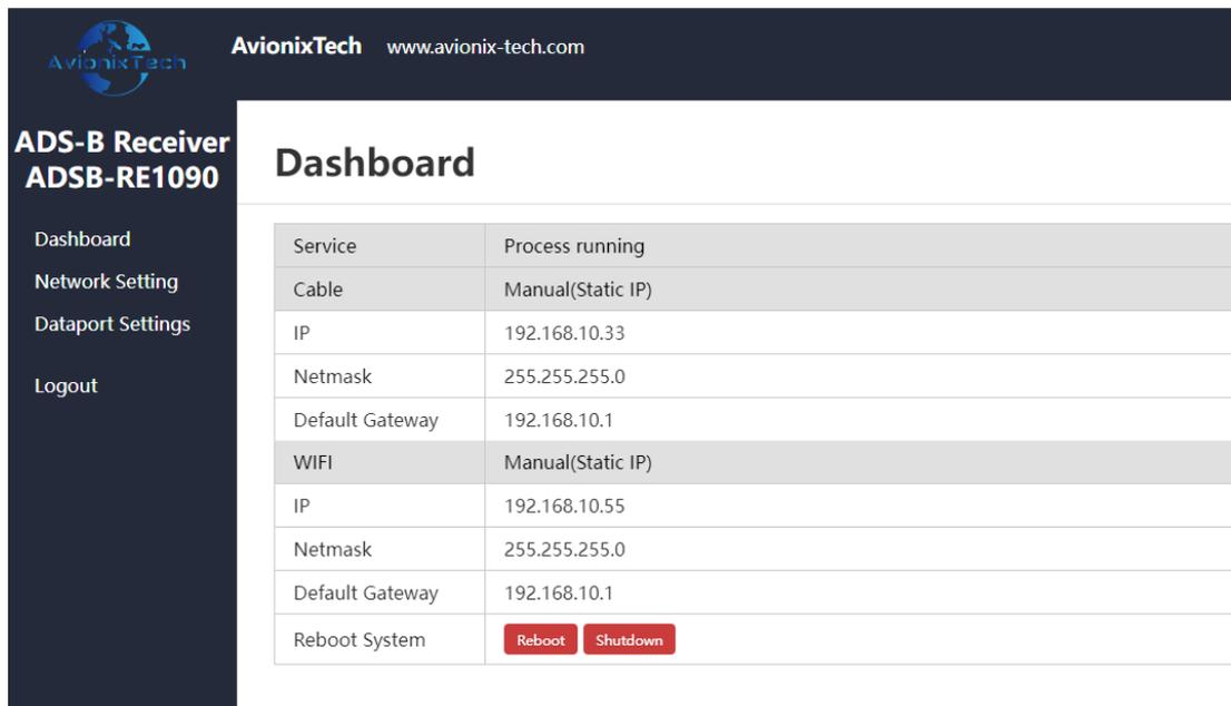
The screenshot shows the AvionixTech website interface for the ADSB Receiver ADSB-RE1090. The dashboard displays network configuration for both Cable and WIFI. The Cable section shows IP: 192.168.10.33, Netmask: 255.255.255.0, and Default Gateway: 192.168.10.1. The WIFI section shows IP: 192.168.10.55, Netmask: 255.255.255.0, and Default Gateway: 192.168.10.1. Both sections are set to Manual(Static IP). A Reboot System section contains Reboot and Shutdown buttons.
