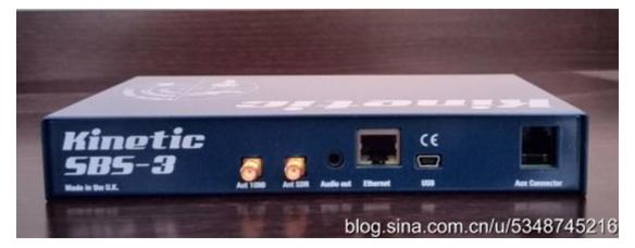
Simple start is to connect SBS-3 with computer via the USB cable and install the BaseStation software on computer. No need for any further configuration, you'll see aircrafts immediately. Computer would power SBS-3 also via the USB cable.
