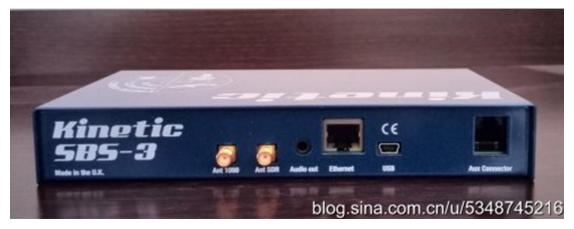
Simple start is to connect SBS-3 with computer via the USB cable and install the BaseStation software on computer. No need for any further configuration, you'll see aircrafts ADS-B information immediately. Computer would power SBS-3 via the USB cable.
