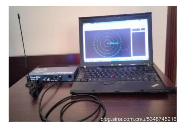
You may be aware that ACARS frequencies are different from country to country. It's not like ADS-B. ADS-B has a global frequency 1090MHz, and U.S.A. general aviation special UAT frequency 978MHz. Let's take ACARS frequency 131.45MHz as an example for showing how to configure SBS-3 to work as an ACARS receiver. In BaseStation software, enter Software Defined Radio Control Panel.
