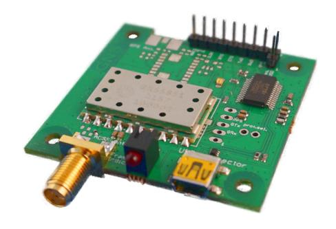
The GNS 5851 StarterKit has been designed to support developers during design-in of the GNS 5851 stand-alone module solution.
