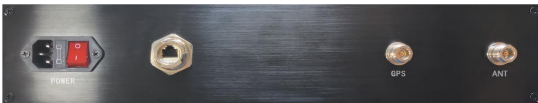
Rear Panel: From left to right – Power Socket, Network Port, GNSS Antenna Port, AIS Antenna Port
